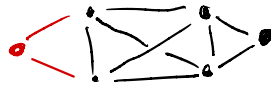
Figure 3: Reducing Eulerian walks to Eulerian tours: after adding the red vertex and edges all degrees are even
