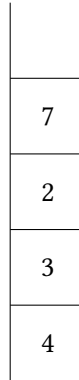
Figure 3: A stack S_0 containing the numbers 4, 3, 2, and 7 (7 is the top of the stack)
